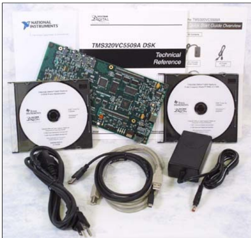
TMS320VC5509A DSP Starter Kit (DSK)
