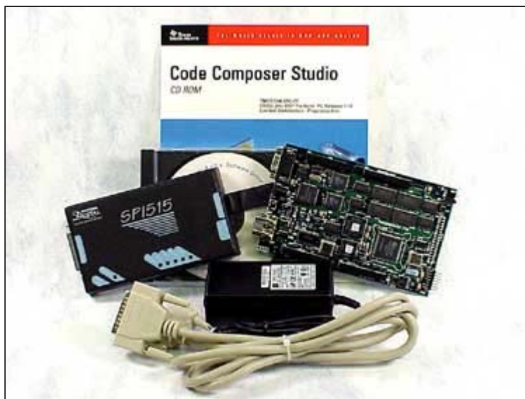
EVM320LC549 + Power Supply + SPI515 JTAG Emulator + Code Composer Studio for the C5xxx
