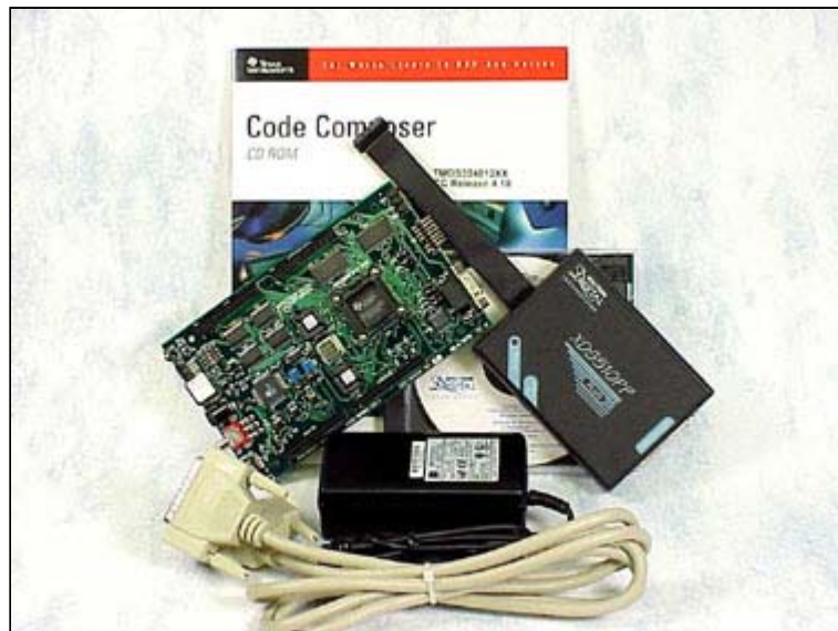
EVM320LF2407 + Power Supply + XDS510PP PLUS Emulator + Code Compos Studio for the C2xxx
