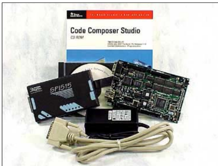
EVM320VC549 + Power Supply + SPI515 JTAG Emulator + Code Composer Studio for the C5xxx
