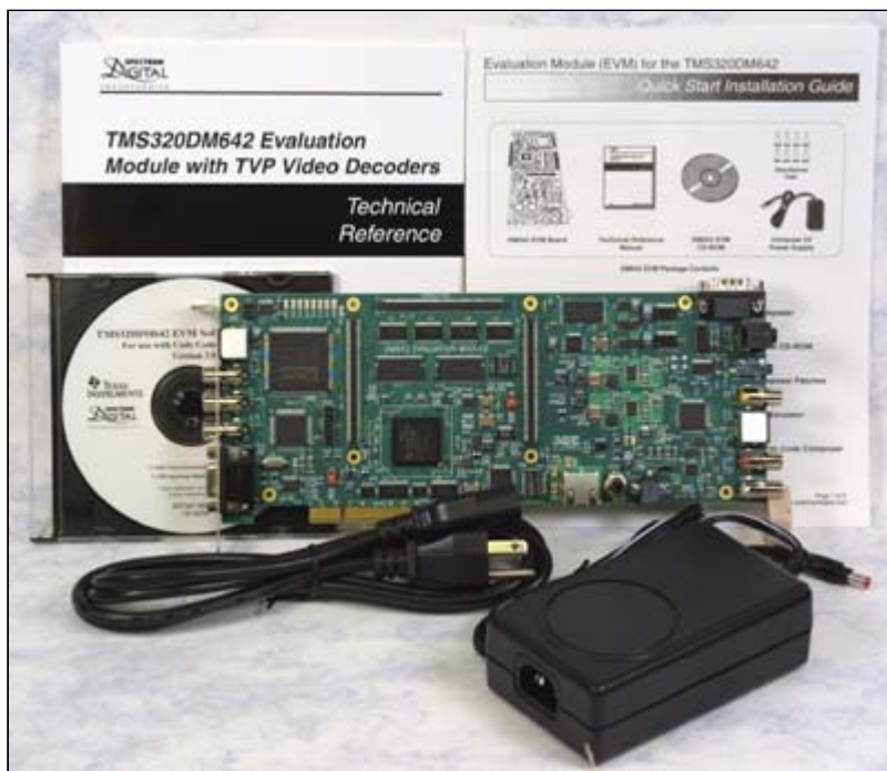
DM642 Evaluation Module with TVP Video Decoders, 720 Mhz.
