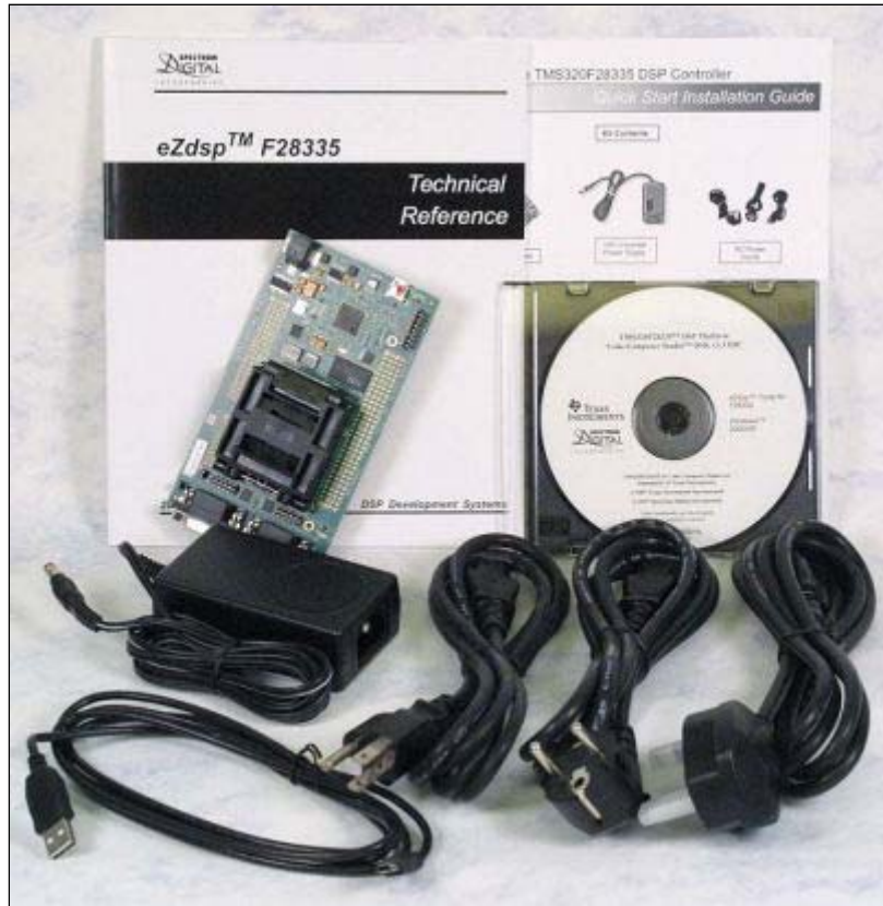
eZdsp™ F28335 board with Code Composer Studio DSK tools and power supply
