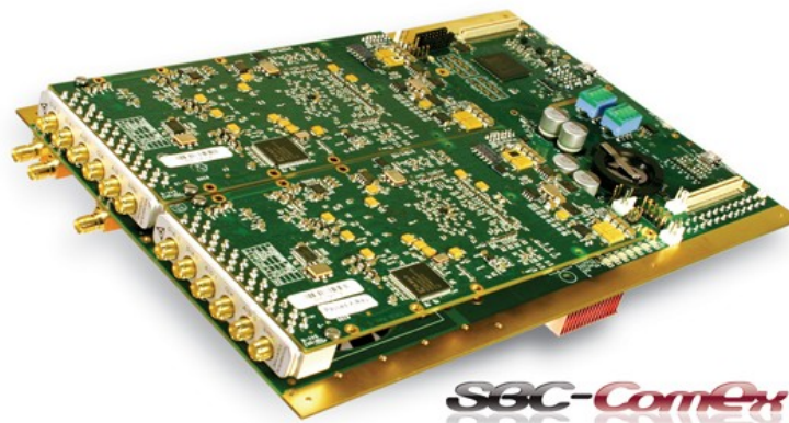
SBC COMEX Motherboard with Two XMC modules
